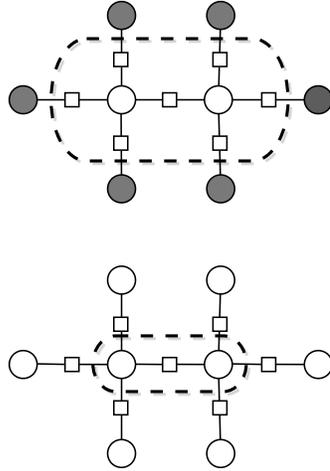
**Figure 4.2.** Schematic factor-graph depiction of the difference between pseudolikelihood (top) and piecewise training (bottom). Each term in pseudolikelihood normalizes the product of many factors (as circled), while piecewise training normalizes over one factor at a time.
