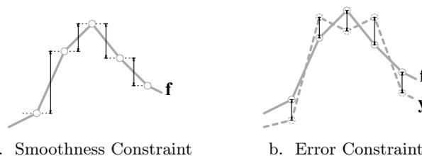
Figure 5. Smoothness and error constraints for a function on a linear graph. In Figure a, the smoothness constraint penalizes functions where neighboring nodes in  $\mathbf{f}$  receive different values. In Figure b, the error constraint penalizes functions where nodes in  $\mathbf{f}$  receive values different from the corresponding values in  $\mathbf{y}$ .
