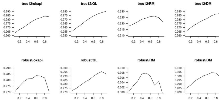
Figure 9. Performance as a function of amount of regularization. For each value of  $\alpha$ , we selected the values for  $k$  and  $t$  maximizing mean average precision. A higher value for  $\alpha$  results in more aggressive regularization. A low value of  $\alpha$  recovers the original scores.
