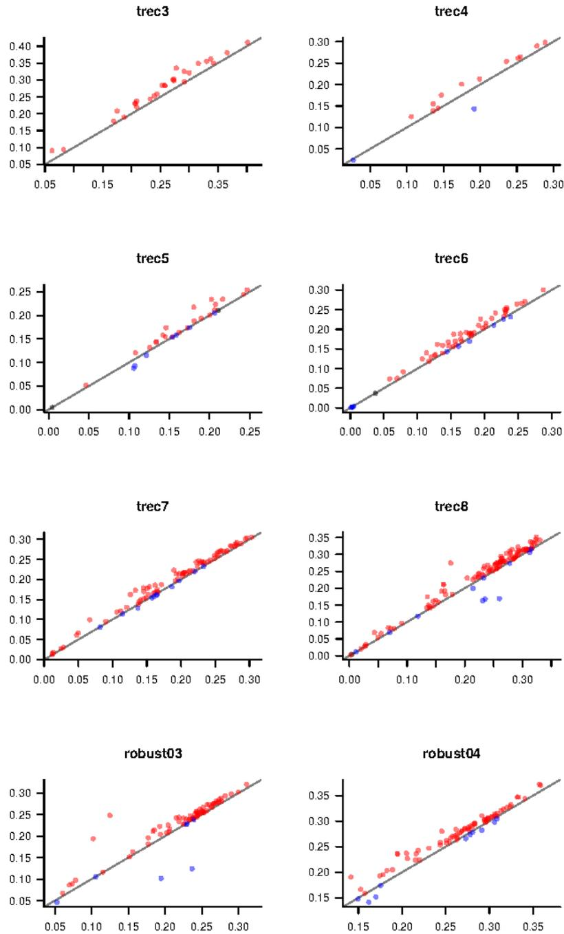
*Figure 11.* Improvement in mean average precision for TREC query-based retrieval tracks. Each point represents a competing run. The horizontal axis indicates the original mean average precision for this run. The vertical axis indicates the mean average precision of the regularization run. Red points indicate an improvement; blue points indicate degradations.
