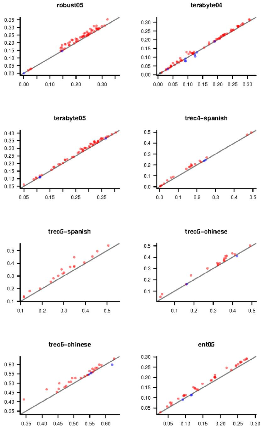
*Figure 12.* Improvement in mean average precision for TREC query-based retrieval tracks. Each point represents a competing run. The horizontal axis indicates the original mean average precision for this run. The vertical axis indicates the mean average precision of the regularization run. Red points indicate an improvement; blue points indicate degradations.
