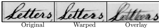
Figure 3: A word image, a resampled version, and an overlay of the two (for comparison).
