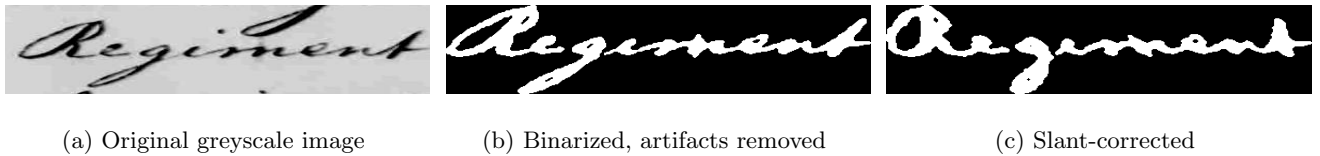
Figure 5: Different processing/normalization steps on a greyscale image of the word Regiment .
