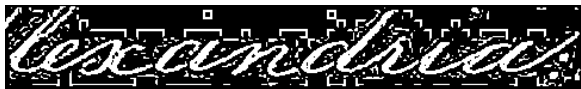
Figure 2: Edge image of an instance of the word Alexandria : JPEG compression artifacts result in “dirt” and phantom edges (e.g. horizontal edges).
