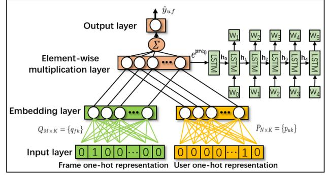
**Figure 5: The framework of text feature modeling.** The preference embedding  $e^{Pr e_0}$  is served as the “Zero State” of a LSTM network, which is further used for generating time-sync comment. The likeness of user  $u$  to frame  $f$  can be simply predicted by conducting logistic function on the inner product between  $p_u$  and  $q_f$ .
