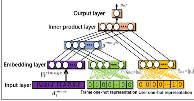
**Figure 4: The framework of image feature modeling.** The preprocessed image feature is merged with frame latent factors to derive a new embedding, which is then multiplied by the user latent factors to generate the prediction.
