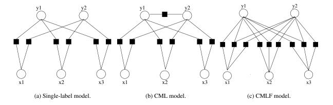
Figure 1: Factor graphs representing the multi-label models, where  $y_i$  is a label and  $x_i$  is a feature, and the black squares represent clique parameterizations. In (a) each parameterization involves one label and one feature. Figure (b) represents an additional parameterization involving pairs of labels, and figure (c) represents a parameterization for each label and each feature, together with each pair of labels and each feature.
