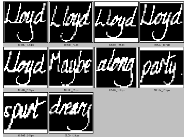
Figure 4: Ranked matches for template ‘‘Lloyd’’ (the rankings are ordered from left to right and from top to bottom).
